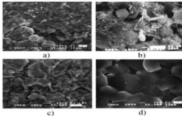
**Figure 9. (a) & (b) Conventional brick (SEM-SE); (c) & (d) Ceramic compound made of a mixture of jal and additive (SEM-SE)**
