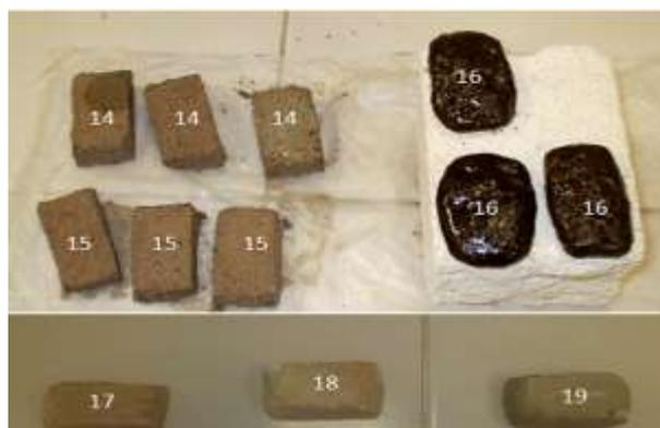
Figure 8. Ceramic compounds made of jal material with addition of expanded perlite and vermiculite
