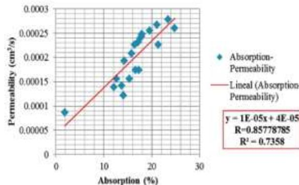
Figure 10. Simple linear correlation between absorption and the permeability
