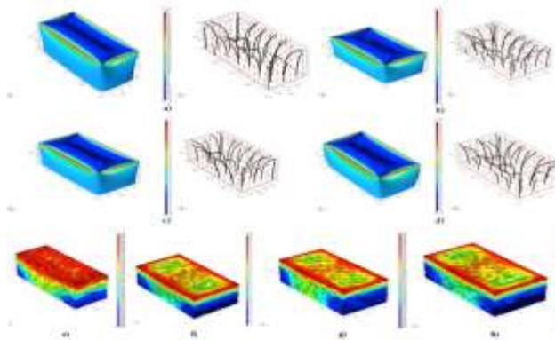
**Figure 14.** (a), (b), (c) & (d) Simulating of Darcy velocity for composites 11, 16, 18 and a conventional brick; (e), (f), (g) & (h) Simulating the compressive strength in the composites 13, 15, 19 and in a conventional brick
