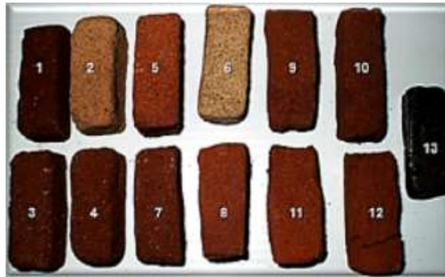
Figure 7. Ceramic compounds made with tailings and clay
