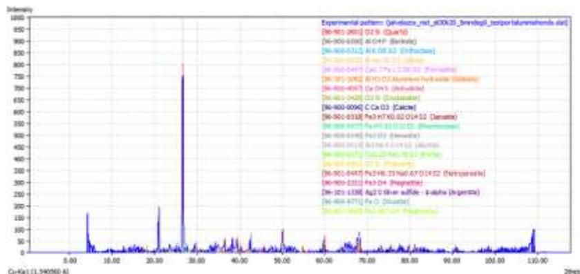
Figure 2. XRD spectrum of the mineral from tailings dam of Velasco
