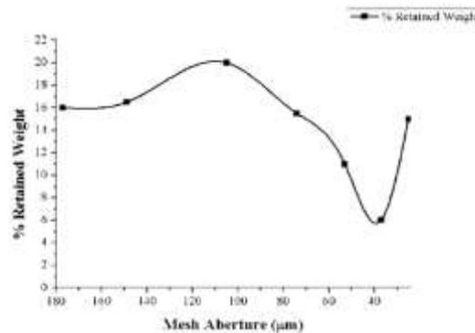
Figure 6. Distribution of particle sizes of the material from Velasco tailings dam
