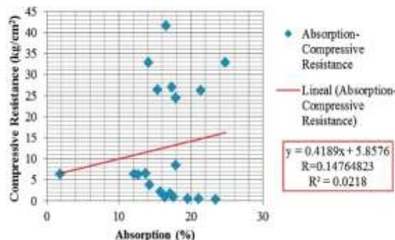
Figure 11. Simple linear correlation between absorption and the compressive strength
