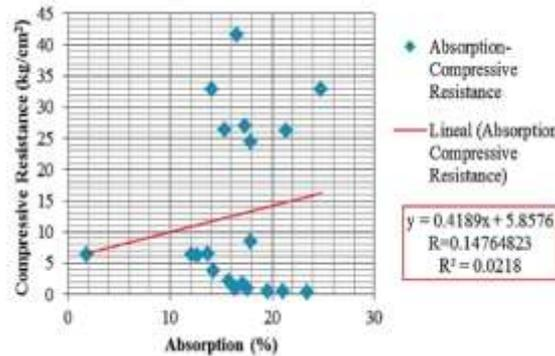
Figure 12. Simple linear correlation between permeability and the compressive strength
