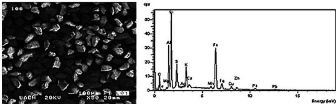
Figure 3. (a) General image of the material from tailings dam "Dos Carlos", retained in mesh 100 (50 x and 20 kV); (b) EDS spectrum taken to the same sample (SEM-EDS)
